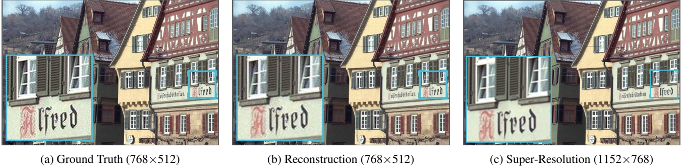
Fig. 2: Demonstration of the super-resolution capability of our learned continuous representation. (a) The original high-resolution ground truth. (b) Our model’s high-fidelity reconstruction at the native training resolution. (c) The super-resolved output generated by querying the same model on a denser coordinate grid.
